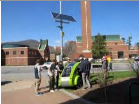
ASU solar charging of ELF
